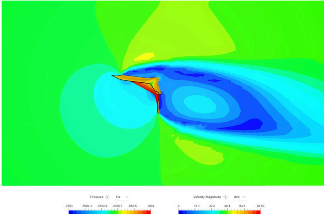
This view illustrates the rear flow structure in a spoiler-less configuration. The low-pressure zone expands significantly behind the car, indicating unstable wake behavior and energy loss.
