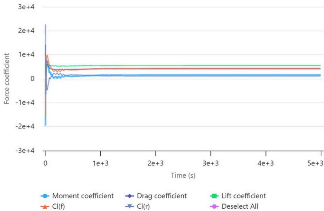
This graph illustrates the time history of aerodynamic force coefficients during the CFD simulation with the ASM spoiler installed. After initial transient fluctuations, all coefficients stabilize consistently.
