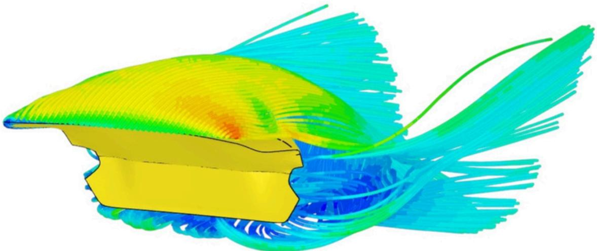
This simulation demonstrates how the ASM dry carbon spoiler significantly improves flow behavior. Streamlines remain attached longer and are deflected downward, showing clear evidence of added downforce. The spoiler directs air in a controlled path, stabilizing the wake and reducing turbulence behind the vehicle. This contributes to the 356 N aerodynamic downforce measured at 140 km/h, improving high-speed stability and grip without excessive drag.
