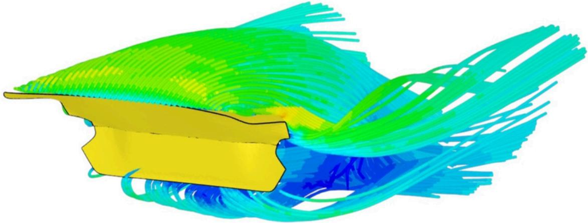
This simulation shows unassisted airflow over the rear trunk of the G87 M2 without a spoiler. The streamlines are more chaotic, with less downward deflection and earlier flow separation. Air passes over the trunk with minimal aerodynamic guidance, producing a wide turbulent wake and reduced downforce. The lack of control leads to lower rear-end grip at high speed and reduced overall aerodynamic efficiency.
