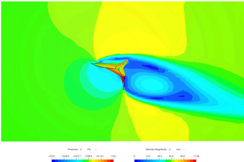
The ASM carbon spoiler compresses and stabilizes the airflow at the rear. The simulation reveals improved pressure distribution and a more organized velocity gradient.
