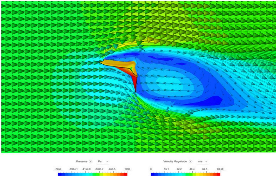
This simulation shows airflow over the rear trunk of the BMW G87 M2 at 140 km/h without any aerodynamic device. The wake behind the car is broad and unstable, with a large low-pressure region (blue) and signs of early flow separation.
