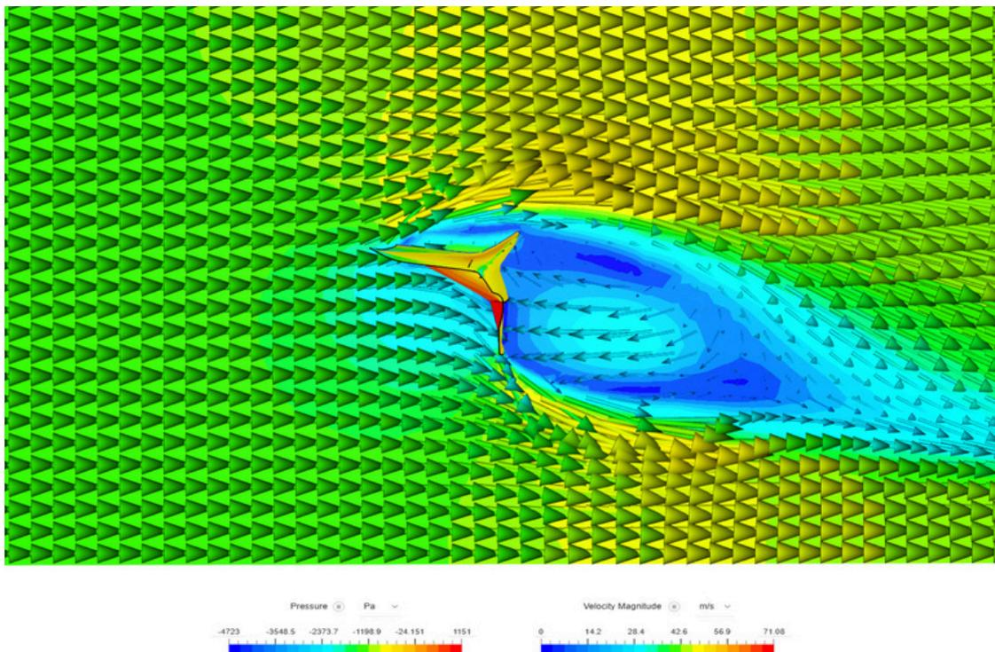
With the ASM spoiler installed, airflow is redirected more effectively over the trunk. The spoiler generates a focused low-pressure zone (dark blue) that increases vertical downforce. The wake becomes narrower and cleaner, showing improved flow attachment and reduced turbulence.
