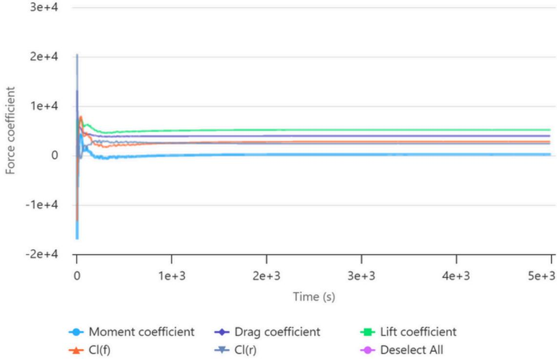
This chart presents the force coefficient evolution over time in the baseline configuration without a spoiler. While convergence is achieved, the overall lift coefficient is lower, and the rear downforce ( $C_{l(r)}$ ) is significantly reduced.
